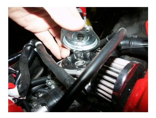
With the plate removed, here's the slide piston spring and diaphragm.
