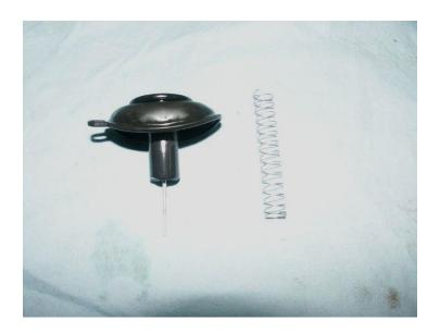
here's a super detail shot of the stock needle position in the slide piston. Notice the little ledge on the needle where it meets the piston:
