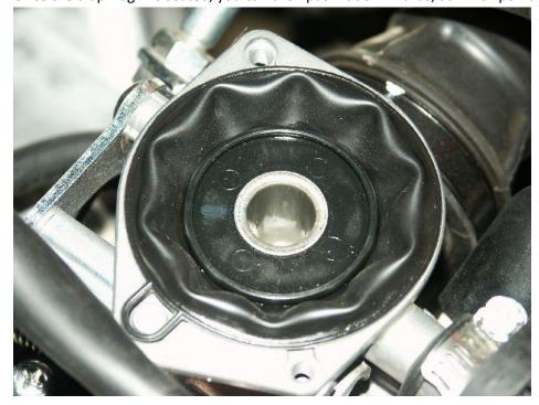
Insert the spring into the top of the piston. Reinstall the plate (make sure the dimple of the plate sits inside the spring) and screw it down into place. Check it from the side to make sure it is sitting flush with the top of the carb. If not, remove it and reseat the diaphragm.
