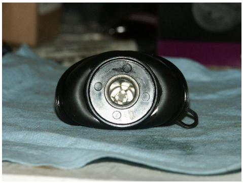
Here's the retainer and needle removed from the piston assembly:
