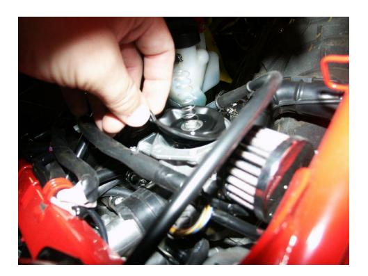
The diaphragm is attached to the top of the slide piston. Hanging from the bottom of the slide piston is the needle. Move over to your workbench and **Do NOT drop this assembly as it could bend/break your needle!**
