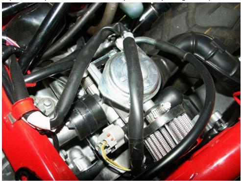
Unscrew the two screws on the top of this plate and very carefully lift it. Notice the spring under the plate.. be very careful to not let this go flying.
