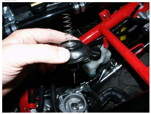
Obligatory overexposed view of the piston spring and slide piston assembly on the workbench:
