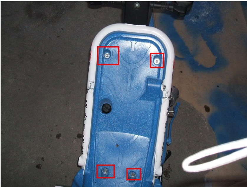
Remove the 8 bolts holding the floorboard on, marked as listed. These are a 10mm socket.
