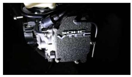
Place new Valve cover over cylinder head. Use 4 of the 5 supplied bolts to fasten valve cover. Place supplied 8 inch hose on Breather nipple on top of the valve cover. If hose is tight use dab of oil on barbed fitting so hose can slide on. Place last bolt through grommet and attach to valve cover. Feed hose through grommet facing down. Tighten
