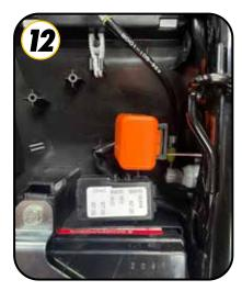
Remove OEM flasher relay. Remove rubber grommet from OEM flasher and transfer to orange (LED flasher relay).
