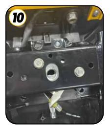
This shows how we ran the wires. You will have a loom going to L and R sides just like OEM. How clean you want to loom to look depends how you route it.
