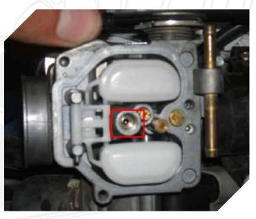
These are a huge pain to take out if you strip the flathead, so please go out and buy the \$10 in screwdrivers and save yourself about 2 hours of work. This is a pic with the main jet removed, just unscrew the old one and screw the new main jet in.
