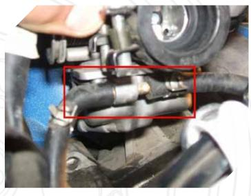
Here's a pic with the coolant hoses connected.... They do flow only one way, and believe us, it's very difficult to connect them opposite.
