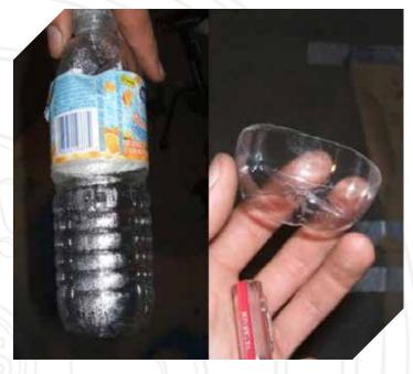
OK! Time to make a gas catcher for when you drain the carb. Just use some water bottle/soda container and chop it down to size. I find these work the best.
