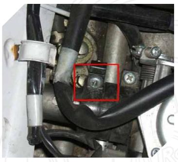
Remove the intake manifold by undoing the screw (PH1), and just wiggle it off (Careful, the intake manifold is hot if you've been riding a little bit.
