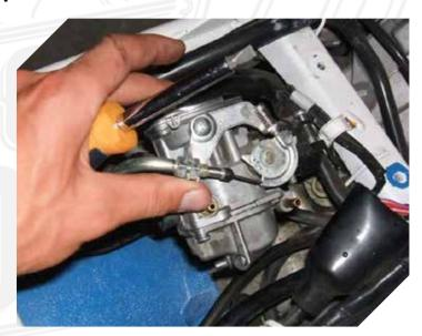
You've now drained the CARB!!! Just rotate it over like shown, remove the two coolant wires (careful, these spit out hot coolant if you've been riding for a while), and flip it over.
