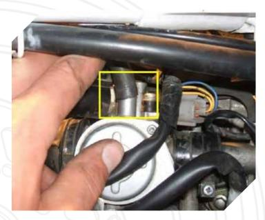
Attach the main hose (red box) back on, tighten the crews on the intake and the main hose (green and red boxes). Attach the secondary vacuum hose (yellow box). That should be everything.
