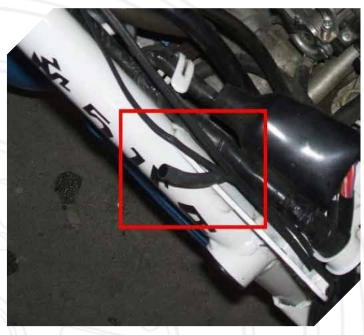
Once you have it removed, just prop it up in between the frame and a couple hoses like shown here to prevent gas from leaking everywhere.
