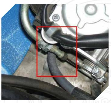
**C)** Remove cable if needed, by loosening the lock nut and sliding out. Most likely you will not need to do this.
