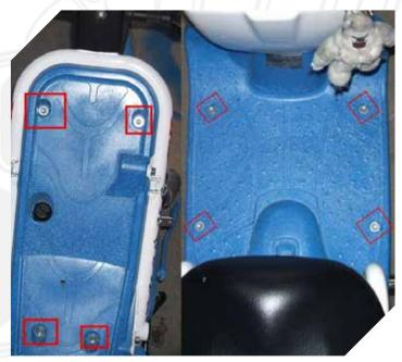
Remove the 8 bolts holding the floorboard on, marked as listed. These are a 10mm socket.
