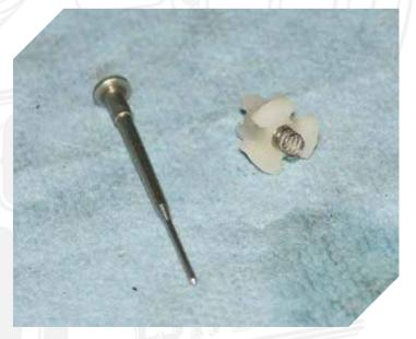
Here's the retainer and needle removed from the piston assembly:
