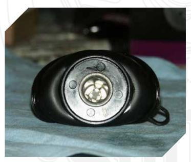
Here is what we need to remove now.. The three sided retainer sits inside the top of the slide piston. Notice the ears inside the piston. There are cams on the retainer that slide underneath to hold it in place. Using the pliers (or a small phillips screwdriver), grab and carefully rotate the retainer counterclockwise. Do not force it. OR USE A 6MM SOCKET AND IT WORKS PERFECT.
