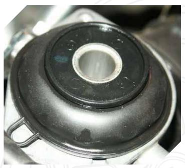
Now time for reinstallation. To reinstall the diaphragm, position it like this and carefully wor the bead of it into its seat on top of the carb.
