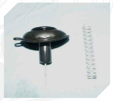
Obligatory overexposed view of the piston spring and slide piston assembly on the workbench.
