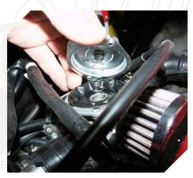
Unscrew the two screws on the top of this plate and very carefully lift it. Notice the spring under the plate.. be very careful to not let this go flying.
