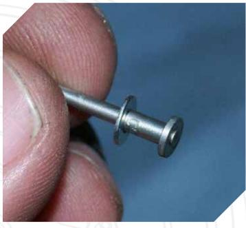
Put the washer on the needle like this. It'll slide allI the way to the base and should seat flush at the end.
