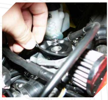
Very carefully lift the little loop and pull the diaphragm up out of its seat in the top of the carb.
