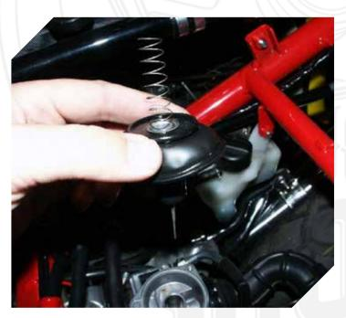
The diaphragm is attached to the top of the slide piston. Hanging from the bottom of the slide piston is the needle. Move over to your workbench and **Do NOT drop this assembly as it could bend/break your needle!**
