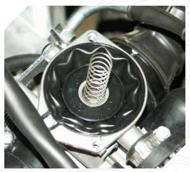
With the plate removed, here's the slide piston spring and diaphragm.
