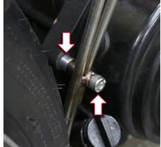
**2.** It's easier to place the exhaust gasket on the studs first. It will align up with the header flange like so.
