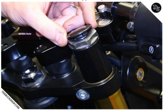
And last but DEFINITELY not least, make sure you re-tighten the upper triple clamp bolt!
