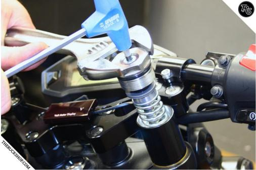
Then, install the top cap back on... you will have to press down a bit to compress the spring... it can help to use the socket to grip the top cap or press down on the Allan-wrench. Be careful <u>NOT</u> to cross thread the nut.
