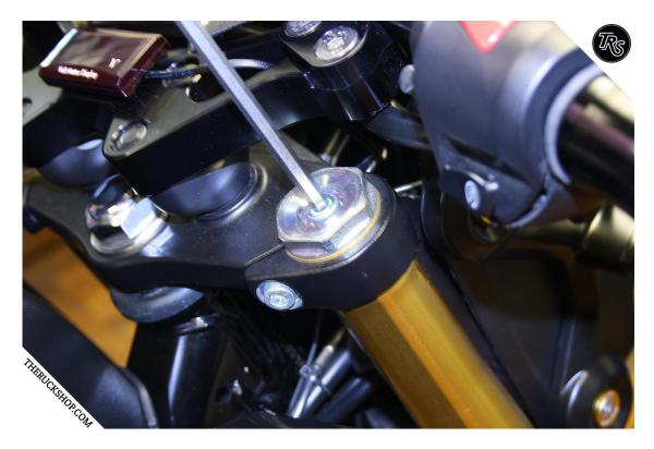
Then, using a 36mm Socket (or open wrench), you'll want to completely unscrew the top cap... The bike will drop down a little bit when it comes loose, since only one fork will now be holding it up. Not to worry, hopefully your friend is helping hold the bike.
