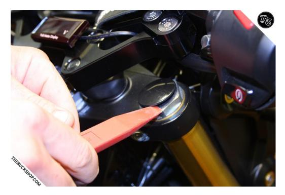
Then, take an allen key, and loosen the top triple tree clamp bolt.
