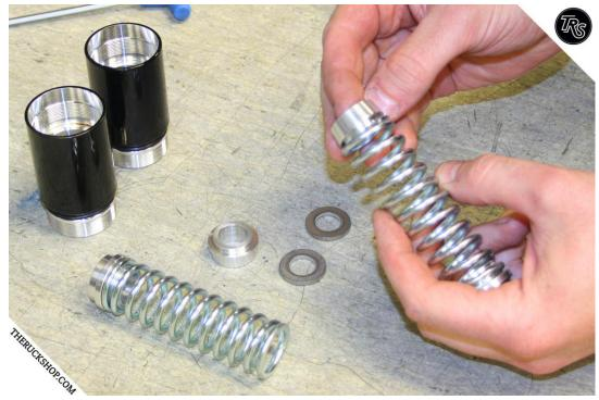
Now, you'll take the spring with the upper and lower seat, and slide them over the damper rod, into the fork tube... make sure that the lower spring seat fits into the top of the fork shaft... if it is off-center, it will not sit correctly on the fork tube!
