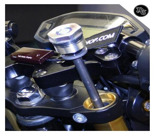
Then, go ahead and unscrew the center bolt all the way, and remove the top cap from the damper rod... you will be left with the top cap, a rubber bump stop, and a large washer. We will not be re-using the washer as a new one is provided, but we will re-install the bump stop
