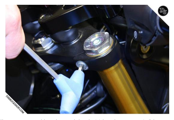
Then, you want to crack loose the center bolt so that it is loose, but not remove it all the way yet.
