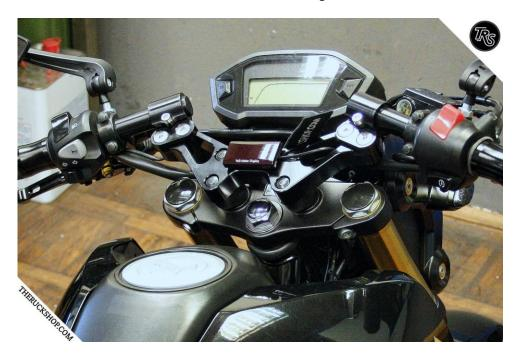
To start with, we removed the stock handlebars. They have little plastic buttons over the bolts. These caps need to be removed. Use a very small flat-head screwdriver to get underneath them, and pry them off. Once off, remove the bolts. Once you have the handlebars off, we normally get a towel to protect the dash, and then drape the bars over the front of the bike. Remember, you will be changing the bars to do this, as the stock bars won't fit once the lowering kit is
