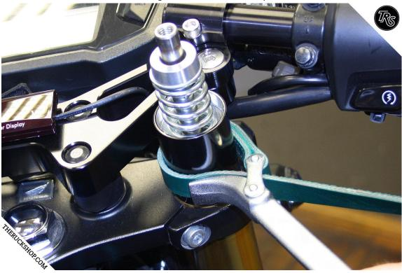
Next up, take the original bump stop and the supplied washer... you will want to install these on the damper rod... first the washer, and then the bump stop.
