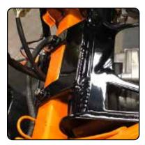
**4.** Bolt on the shock extension bracket and the shock. Some medium strength (blue) threadlock is useful here.
